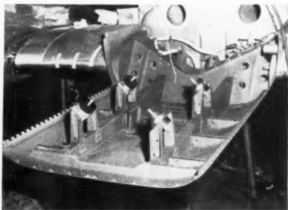
PARALLEL MOUNTED nacelles mean less cross sectional drag, and their top surfaces generate 12% of total lift. Engines are mounted on built-up sheet metal structures (right). Heavy rubber biscuit-type mounts reduce vibration transmission.
